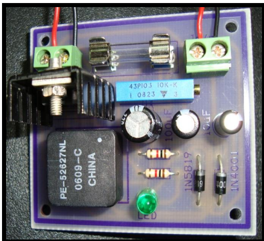
Fig 4: Photograph of top view of the Linear Current Booster circuit prototype
