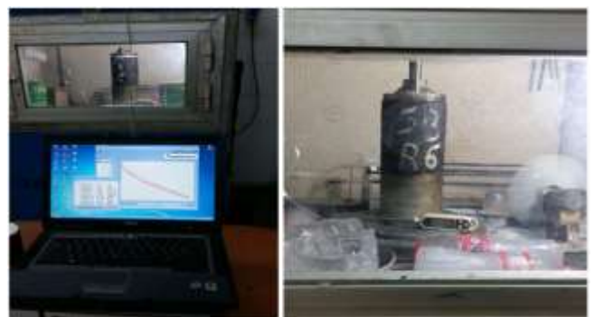
Fig 4: Repeated compressive stress in the PRLS
