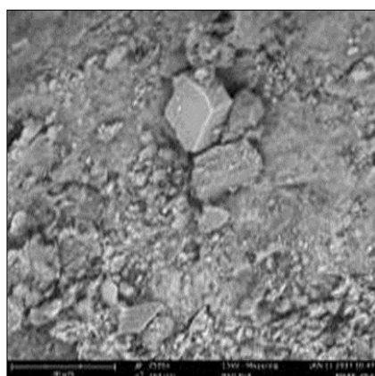
Plate 4.6: SEM of 20% PSA Replacement
